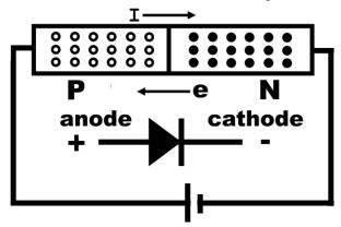
and electron flow. If the charge on the Anode is more positive than the charge on the Cathode, electrons will be pulled from the N crystal and into the holes in the P crystal. We have current flow through the diode. This is called **Forward Biased**. What would happen if the Anode were more negative than the Cathode? The more positive charge on the N crystal would try to pull electrons from the crystal, but there is no way
